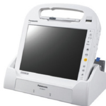
Figure 3: Mobile IP65-certified tablet with integral bar code scanner for mobile EM workflow execution. Workflows are presented to the operator with compliance checks for media/materials, devices and instruments supporting “right-first-time” execution.
