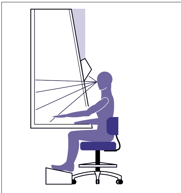
Figure 4 SterilGARD® III Advance®. The SterilGARD® III Advance® biological safety cabinet includes many ergonomic design features which can improve worker comfort and productivity. (The Baker Company)
